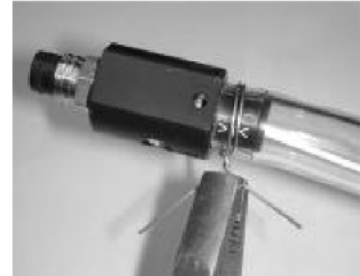
NEATLY WRAP, TWIST & TRIM SS WIRE, FOLD SHARP END INWARD
