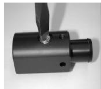
INSTALL GREASE FITTING (NOTE: TOP OF FITTING MUST BE WITHIN PART DIAMETER)
